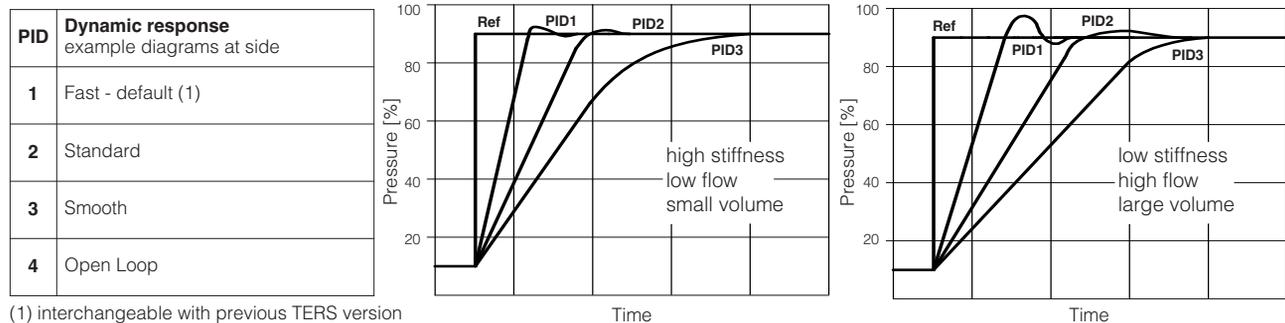
Above indications have to be considered as a general guideline, being affected by hydraulic circuit stiffness, working flow and dead volume. The valve's dynamics can be further optimized on the specific application, customizing PIDs parameters.
