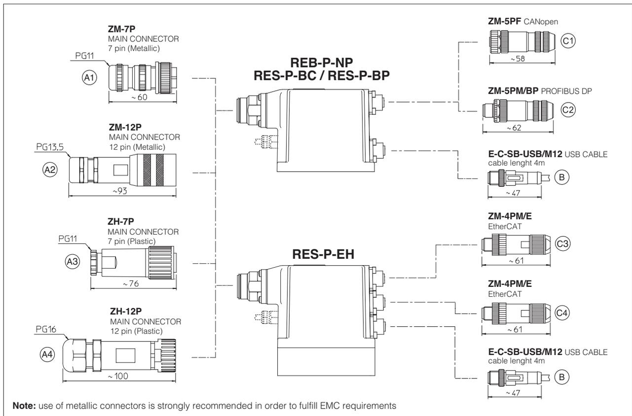
17 MODEL CODES OF MAIN CONNECTORS AND COMMUNICATION CONNECTORS - to be ordered separately
