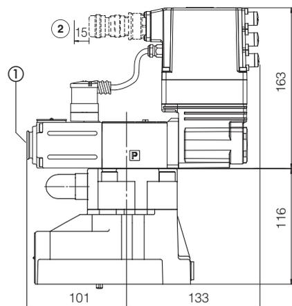
① = Screw for air bleeding: at the first valve commissioning the air eventually trapped inside the solenoid must be bled-off through the screw ①
