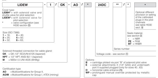
Note: for the code of the ISO cartridge to use with the above covers see tab. H003, section 2 and tab. H030, section 3 (1) Not for multicertification M group I (mining)
