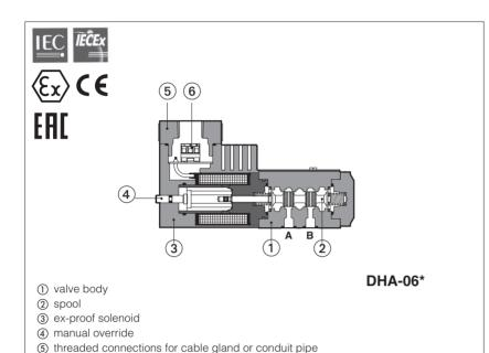
On/off valves equipped with explosion-proof solenoids available with following multicertifications:
