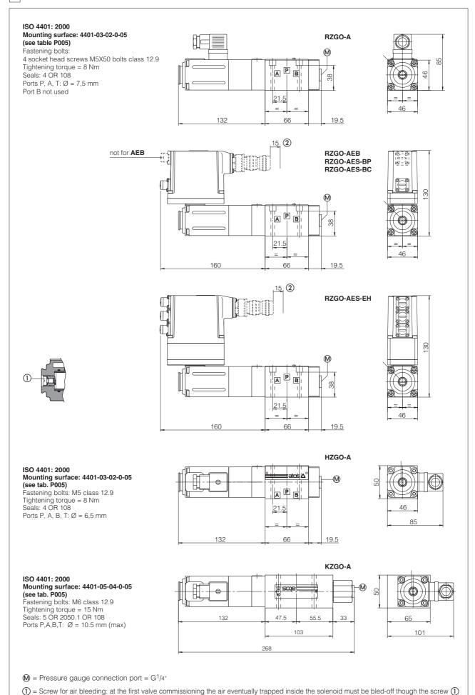
(2) = Space to remove the 7 or 12 pin main connector. For main and communication connectors see section 12, 13
