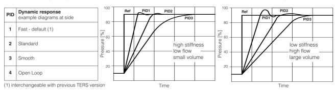
Above indications have to be considered as a general guideline, being affected by hydraulic circuit stiffness, working flow and dead volume. The valve's dynamics can be further optimized on the specific application, customizing PIDs parameters.
