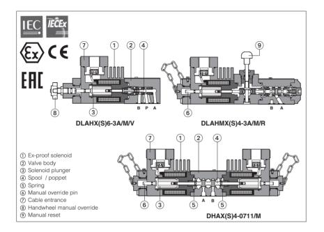
New line of directional solenoid valves and pressure relief valves in stainless steel execution for corrosive environments. Ex-proof Stainless steel solenoids ①, with **ATEX, IECEx, EAC Multicertification** or
