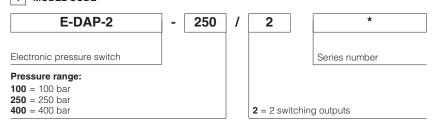
E-DAP-2 is a compact electronic pressure switch with integral digital display, available for 3 different pressure ranges.
