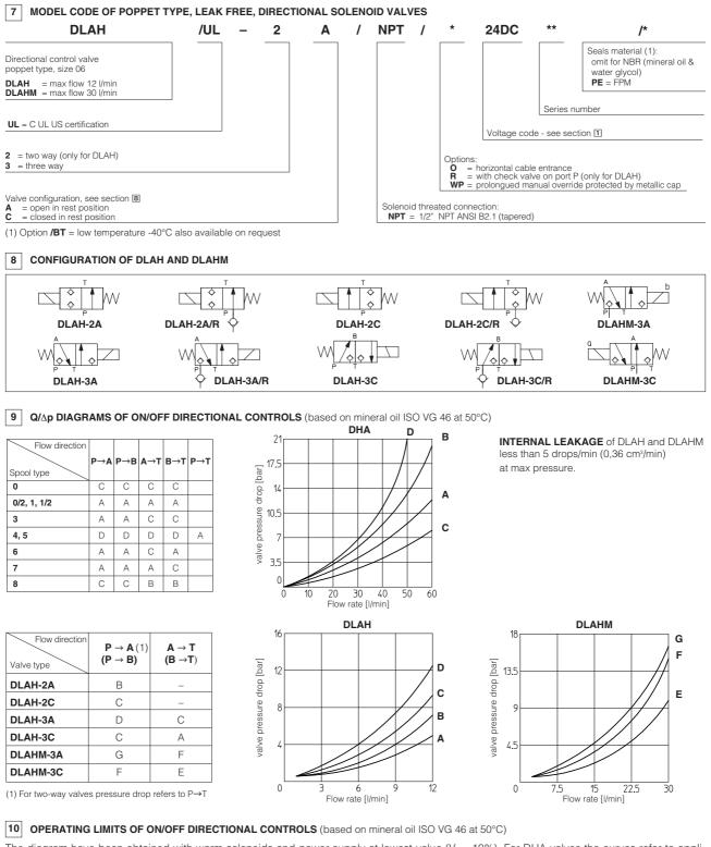
The diagram have been obtained with warm solenoids and power supply at lowest value ( $V_{nom}$ -10%). For DHA valves the curves refer to application with symmetrical flow through the valve (i.e. P  $\rightarrow$  A and B  $\rightarrow$  T). In case of asymmetric flow the operating limits must be reduced.
