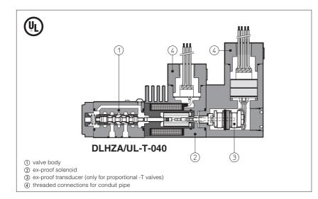
Explosion-proof on/off and proportional solenoids certified cULus according to UL 1002 and CSA 22.2 nº139-1982 Standard, Class I, Groups C&D (Groups IIA & IIB to NEC 505-7).
