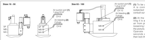
(1) To be used only in case port A is connected to tank and subjected to negative pressure, consult our technical office.
