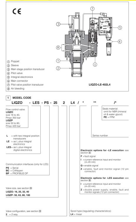
LIQZO-L\* and LIQZP-L\* are 2-way proportional cartridge valves, with double position transducer designed for mounting in mainfold blocks which provide proportional non compensated flow control according to electronic reference signal.
