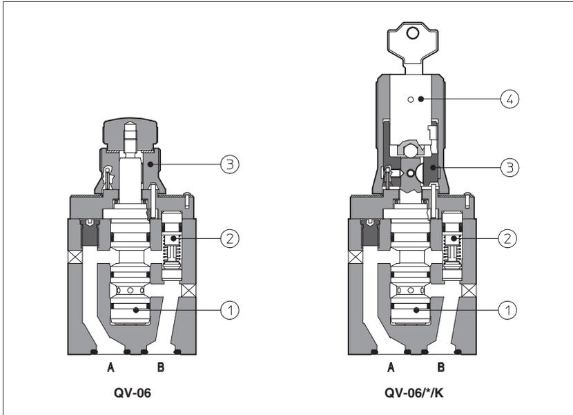
**QV** are flow control valves with pressure compensator (1): the controlled flow rate is independent of pressure variations.
