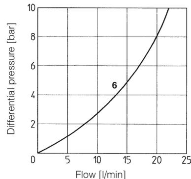
**4.2 Q/Δp diagram through the check valve for free flow B→A**
