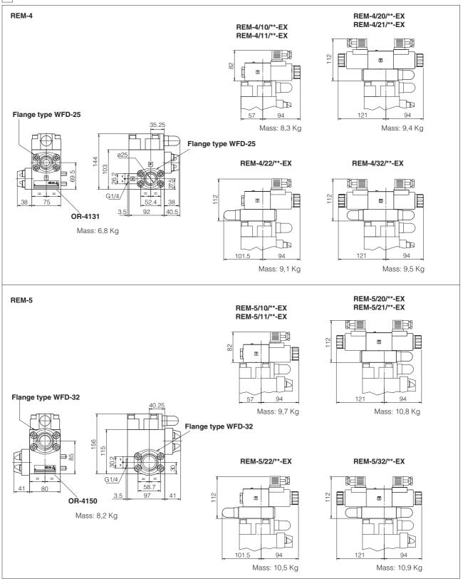
Overall dimensions refer to valves with connectors type 666
