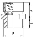
The breather plug with valve proposed here works on the following principle: venting is obtained by the pressure inside the reducer acting on the closing gasket, which raises the spring preset to a pressure of 0.25 - 0.30 bar allowing the vapours to escape and then closes.
