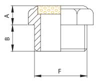
The silencer cap with sintered pad condenses the vapours present, making them fall back inside the tank. - Body in brass OT 58.
