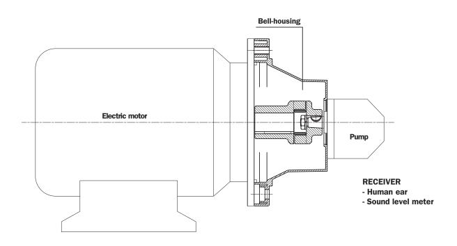
The electric motor and the pump, together with the drive coupling, are the SOURCE OF THE NOISE.
