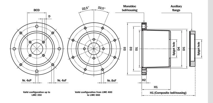
The auxiliary flange, if specified, is supplied already fitted to the bell-housing (MODUL-2).
