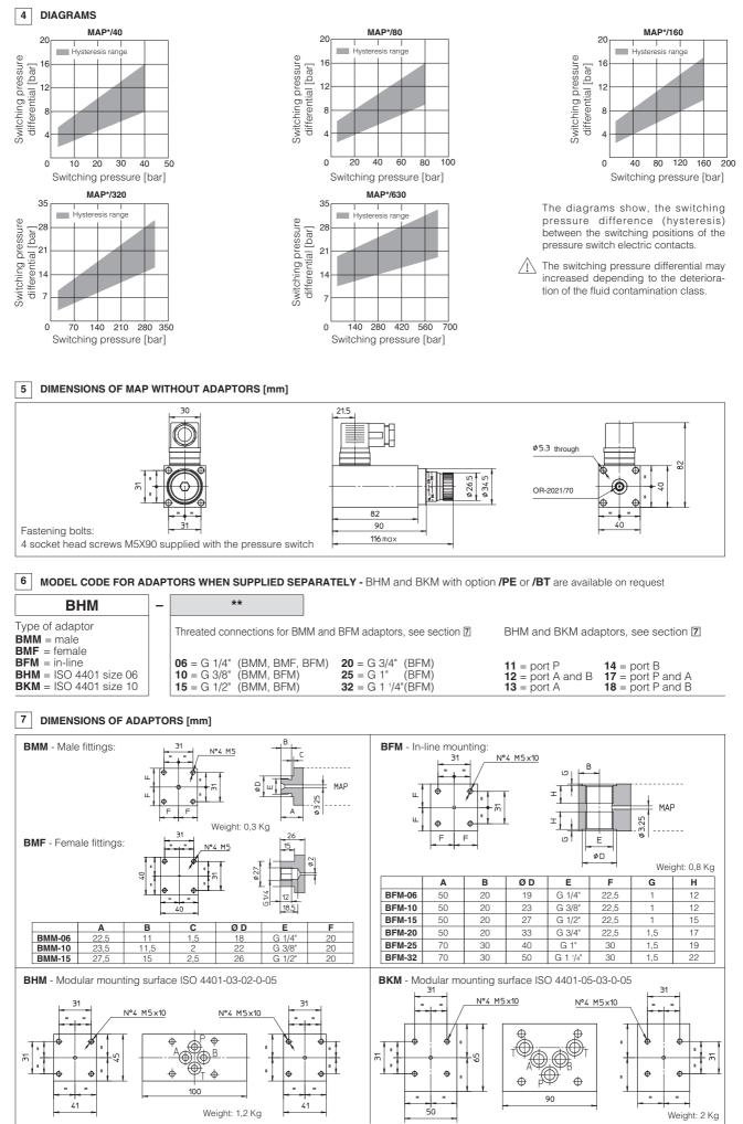
For versions 11 and 13 the pressure switch is mounted on side of port A. For version 14 the pressure switch is mounted on side of port B. For versions 12, 17, 18 the pressure switch is mounted on both sides.
