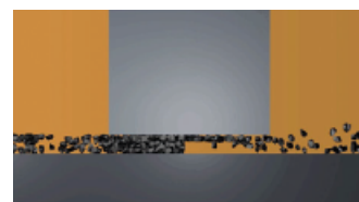
CONTAMINATION IN PRESENCE OF NARROW TOLERANCES
