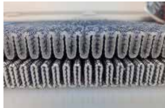
The Filter Media has absorbed water
