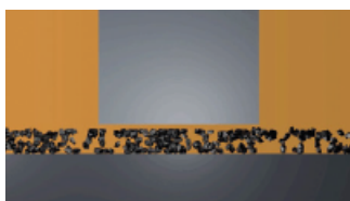
CONTAMINATION IN PRESENCE OF LARGE TOLERANCES
