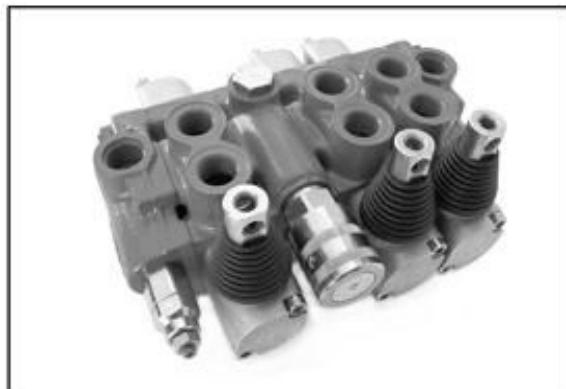
The motor (A) is fed by the whole flow of the pump (P). The cylinders (C, D) downstream the flow control element (RFS) are fed only by the priority flow (PF) which is adjustable through the flow control knob on the element.
