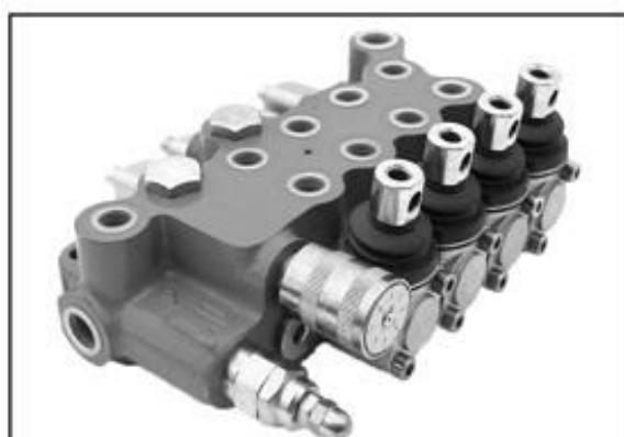
All cylinders (B, C, D, E) are fed by the priority flow (PF) which is adjustable through the flow control knob on the directional control valve. The exceeding flow (EF) is recuperated so that it allows the contemporaneous usage of another valve by adding a CO plug.
