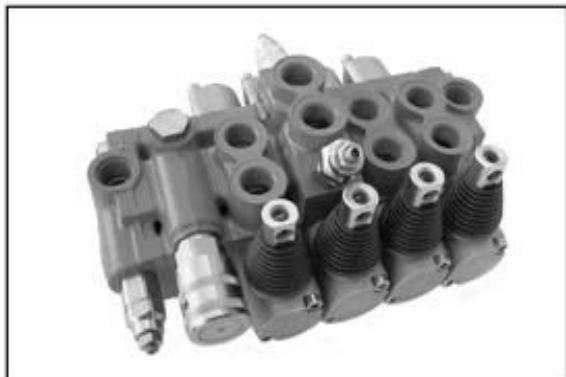
The motors (A, B) are fed by priority flow (PF) which is adjustable through the flow control knob on the element. The cylinders (C, D) are fed by the whole flow of the pump (P) when singly actuated. When a cylinder and a motor are simultaneously actuated, the motor is fed by a priority flow (PF) and the cylinder by the exceeding flow (EF). If a cylinder is actuated while a motor is in work, this last will not vary its rotation speed.
